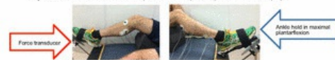
Figure 3. Experimental set up. Six recording EMG electrodes were affixed to all three heads of the triceps surae. EMG and muscle force were continuously measured during MVC and throughout the muscle cramp.
